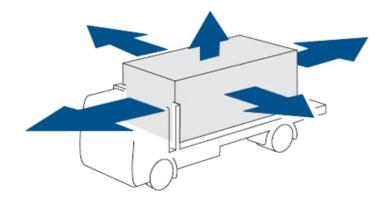
Loads should be restrained from moving in each direction.
