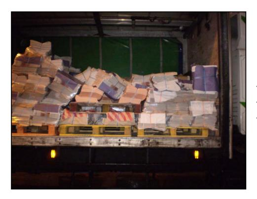
Even if the curtain stops the load falling out during transport, there is nothing to stop the load shifting inside the trailer
