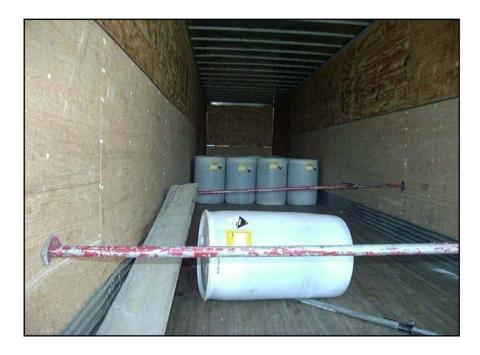
These containers are contained within the vehicle body but are still free to move relative to the trailer bed.
