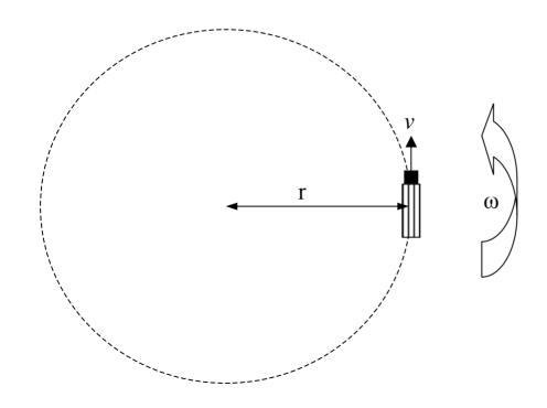
A vehicle going round a corner is in fact travelling around an imaginary circle with a radius, r.
