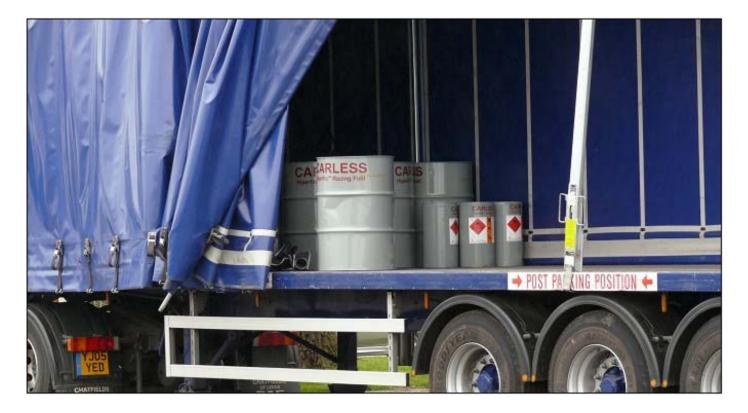
On a curtain sider, closing the trailer curtain and hoping for the best is not transporting a load safely!
