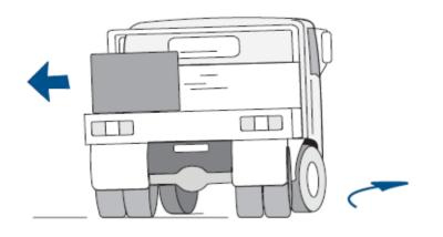
Load shifts on the road can increase the chance of rollover, particularly on roundabouts and motorway slip roads, and when cornering.
