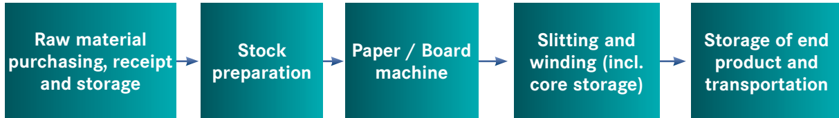
Figure 5 – Flow Chart for Papermaking Process
