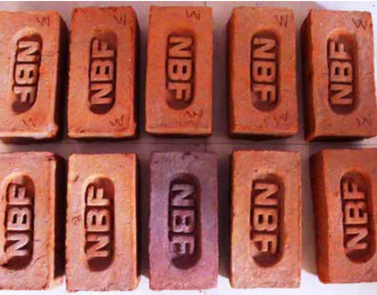
Bricks produced using paper mill sludge
